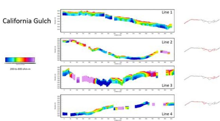
Example of electromagnetic data - blue shows highly conductive zones where subsurface water may be in connection with or close to the stream.
